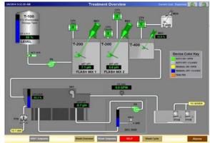
**Operator Friendly Navigation Display** – The Control System operator screens are easy to follow and provide complete system operation and data. Screens are easy to follow and explore with the simple touch of a screen button. You never get lost.
